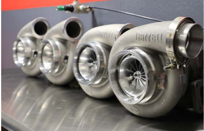
The turbochargers tested are the GTX5020R Gen II 76mm, 80mm, 88mm, and the GTX5533R Gen II 94mm. Tuning is performed by Mark Luton using Fuel Tech software.
