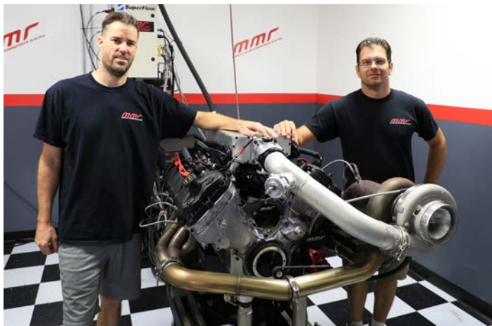
Mark Luton (left) and Greg Seth-Hunter (right) inside the MMR dynocell. The Superflow dyno allows them to test components for performance gains without having to take the racecar to the track.
